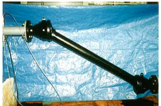
Inspecting of water head loss of TAI-FLEX at each installation condition DN80mm WFF type Bent 27°
