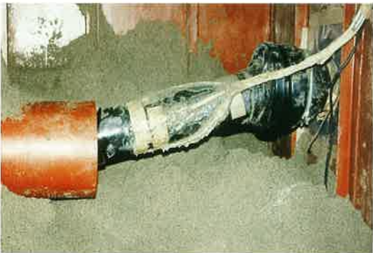
Inspecting of earthquake resistance of underground TAI-FLEX Subsidence 200mm DN150mm WFF-type
