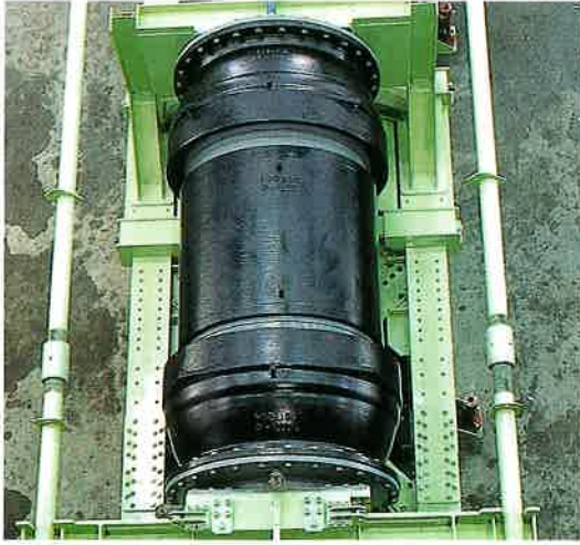
Inspecting watertightness of TAI-FLEX at straight and horizontally. Watertightness test for straight and horizontally installation and repeating test for elasticity DN1200mm
