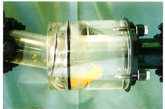
Inspecting water flow inside of TAI-FLEX Flow speed 0.08m/sec. DN80mm
