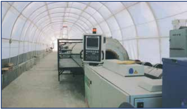
Picture 1.1.12 - A mobile pipe production facility.
