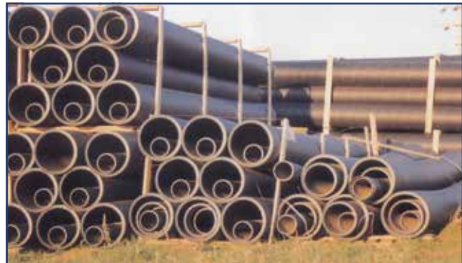
Picture 1.1.9 - Telescopic storage of PE pipes.
